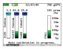
Continuously displays detected isotopes, class, and dose rate for physics-oriented user.
