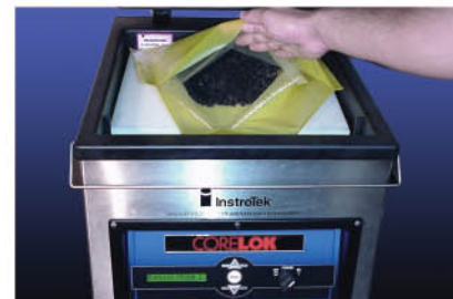
Just place the sample in the bag and place it into the CoreLok. Close the door and the vacuum operation automatically begins.
