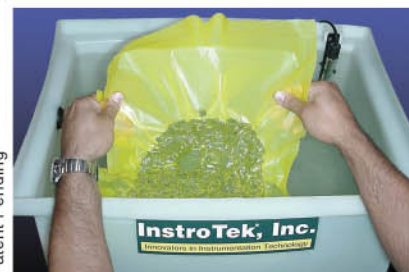
Submerge and cut the bag in water. Allow the scale to stabilize.
