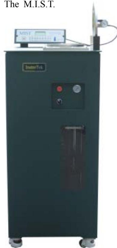
securely fastened . The tank is filled with water; the lid is placed on the tank and heated to 60°C. The sample in the tank is stabilized to 144 °F. The total heating and stailization time is 3.5 hours. Once temperature equilibrium is achieved, the unit begins pressurizing and depressurizing the sample inside the testing tank. This is achieved by the hydraulic cylinder driving the pneumatic cylinder alternately compressing and decompressing the air contained in the cylinder and bladder.
